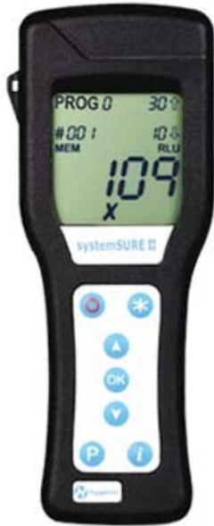
Clearing performance can be quickly assessed with the Bioluminometer.
