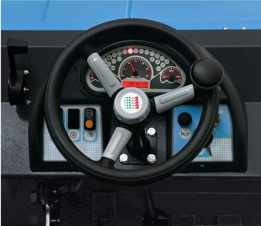
FS80-90-110 have adopted a new, automotive-style design for their instrument panel, with immediate visualisation of all functions. The newly steering wheel has been specially designed for greater comfort when driving. The control panel also features the electric shaker, directly controlled by a button on the instrument panel, which allows the suction pocket filter to be kept clean.
