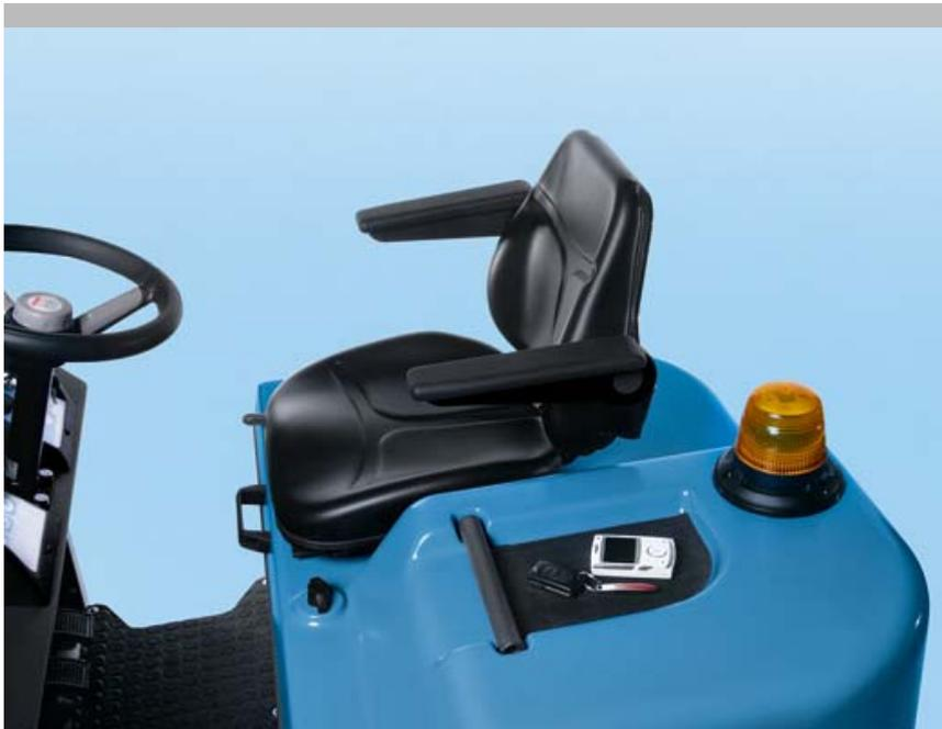
The driver's seat has been carefully devised to ensure the most comfortable operating conditions for the operator: the steering wheel comes with adjustable inclination just like the seat back and the arm rests.
