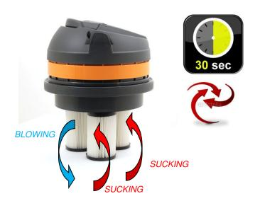
The vacuum cleaner is provided with 3 motors, each one fitted with their own independent filter. The machine works automatically with 2 suction motors and 1 motor idling; when this motor is not working, relevant filter undergoes a cleaning process. Thanks to the motor operation cycles, all the filters get cleaned in turn allowing the vacuum cleaner to work continuously — without losing suction power — with no need of the operator's intervention and providing an efficiency increase.
