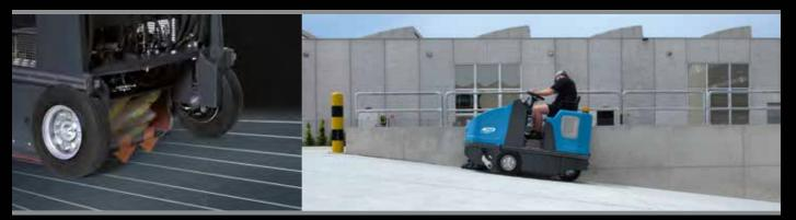
The central brush is the floating type and self-adjusts to keep in contact with the ground all the time
