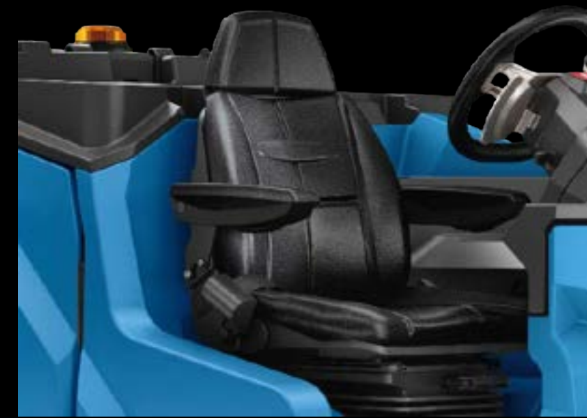
The Comfort seat is adjustable and complete with armrests and safety belt
