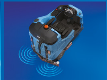
Anti-collision system (rear)
