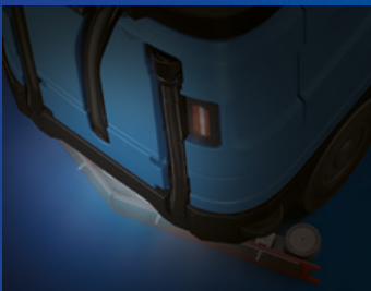
LED service lights
