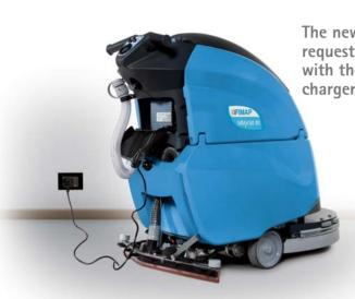
The new Maxima, on request, can be supplied with the on-board battery charger
