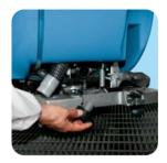
Thanks to the special position of the solution filter cap, water can fully drain away without any water stagnation
